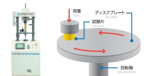
pin-on-disk testing machine
